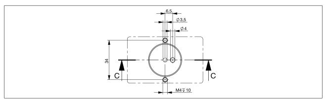
Fig. 7: Connection diagram 2 for plug-in flange variant FC22
