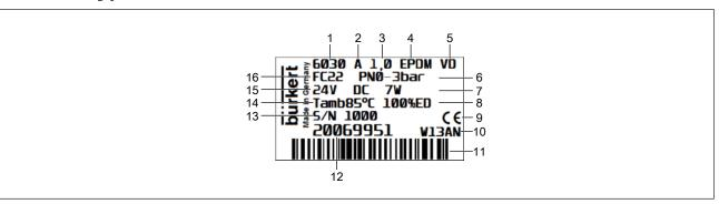
Fig. 4: Type 6030 type label (example)
