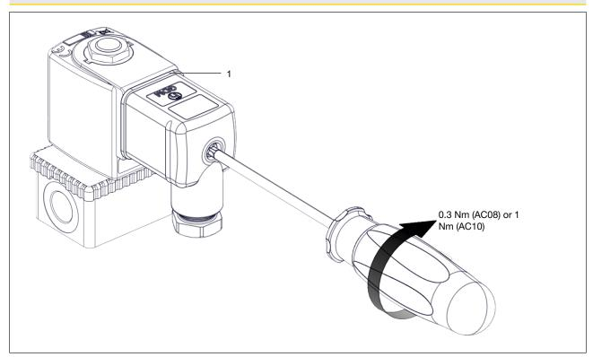
Fig. 14: Install the cable plug
