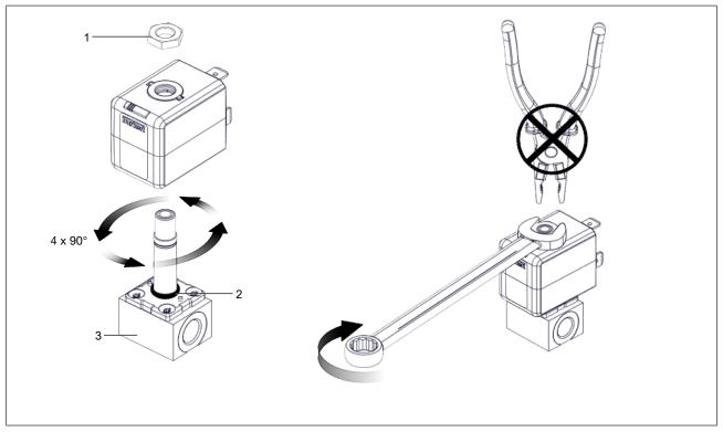
Fig. 13: Coil installation
