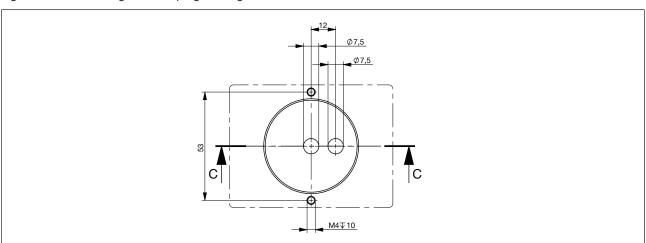
Fig. 9: Connection diagram 2 for plug-in flange variant FC23
