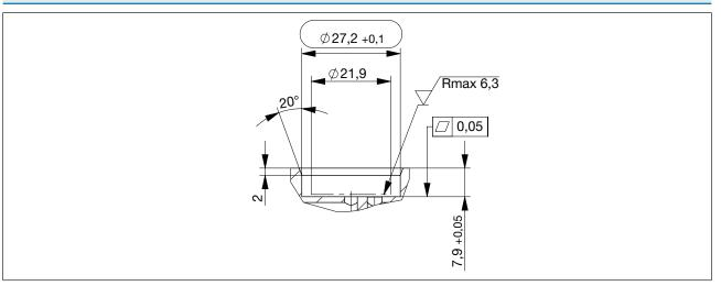
Fig. 6: Connection diagram 1 for plug-in flange variant FC22
