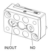
Fig. 2: 2/2-way valve, normally open
