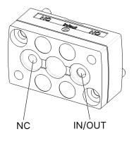
Fig. 1: 2/2-way valve, normally closed
