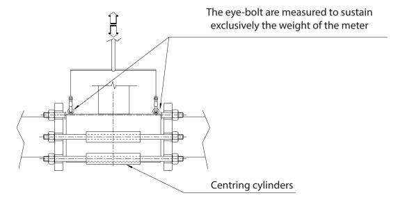
N.B.: For sensor S054 we recommed the use of centring cylinders
