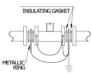
If the sensor has to be mounted on a pipe made of an insulating material is necessary:
