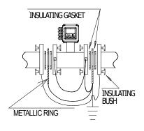
If the sensor must be install in the piping with a chatode protection, is necessary:
