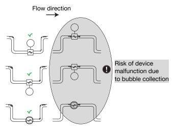
Fig. 24: Horizontal mounting positions
