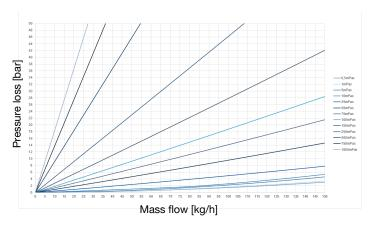
Fig. 23: Pressure loss diagram for DN2
