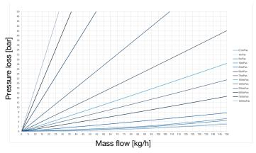
Fig. 19: Pressure loss diagram for DN2
