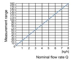
Fig. 14: Measurement range depending on nominal flow rate
