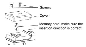
Fig. 32: Insertion direction of the memory card
