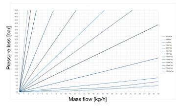
Fig. 22: Pressure loss diagram for DN1
