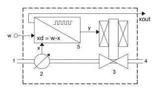
Fig. 31: Function diagram of the MFC with control valve
