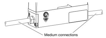
Fig. 34: Medium connections, for example internal-threaded connections
