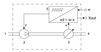
Fig. 30: Function diagram of the MFC with pump
