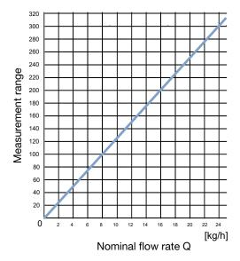
Fig. 15: Measurement range depending on nominal flow rate
