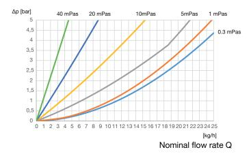
Fig. 21: Pressure loss diagram, MFC with proportional valve
