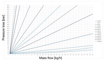
Fig. 18: Pressure loss diagram for DN1
