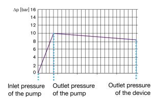
Fig. 20: Pressure loss diagram for water at 20 °C through an MFC with pump
