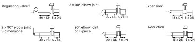
If the valve cannot be mounted after the measuring device, the minimal distances have to be respected.
