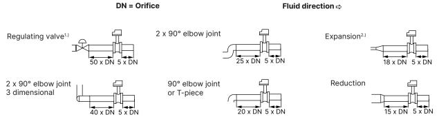
If the valve cannot be mounted after the measuring device, the minimal distances have to be respected.
