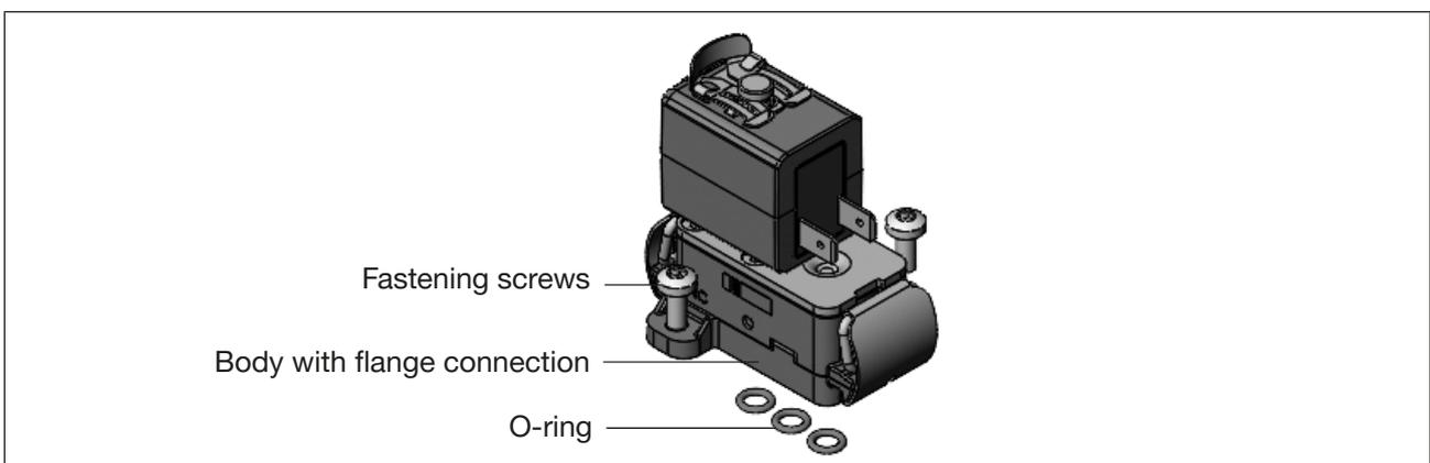
Fig. 7: Installation of devices with flange connection
