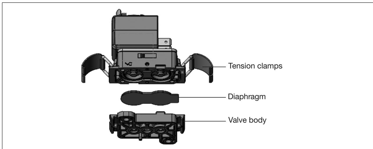
Fig. 10: Replacing the diaphragm
