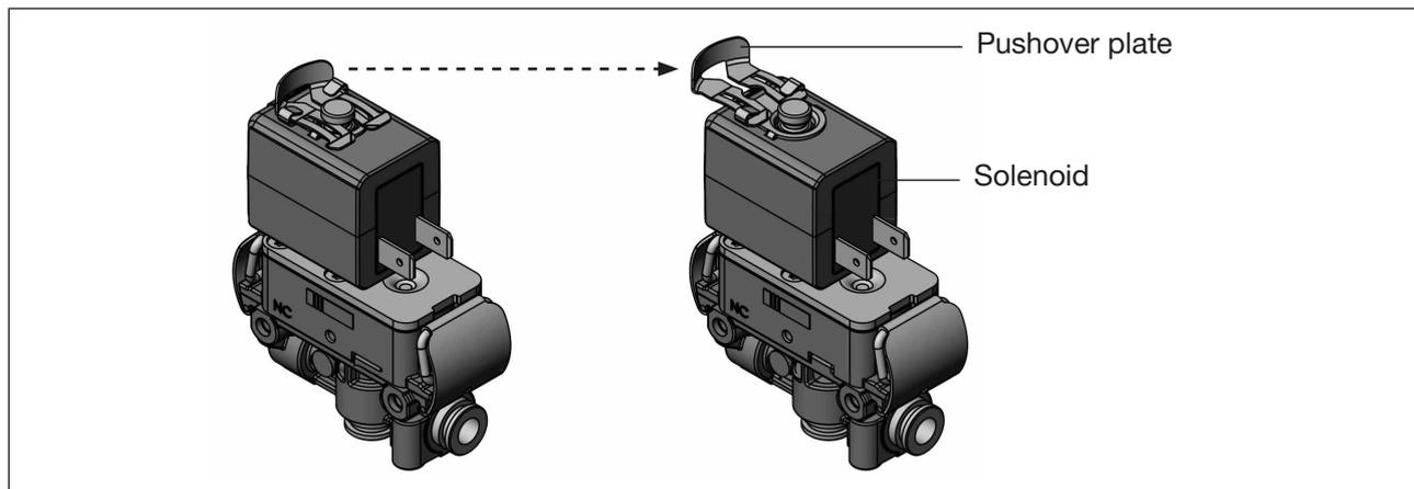
Fig. 8: Loosen pushover plate
