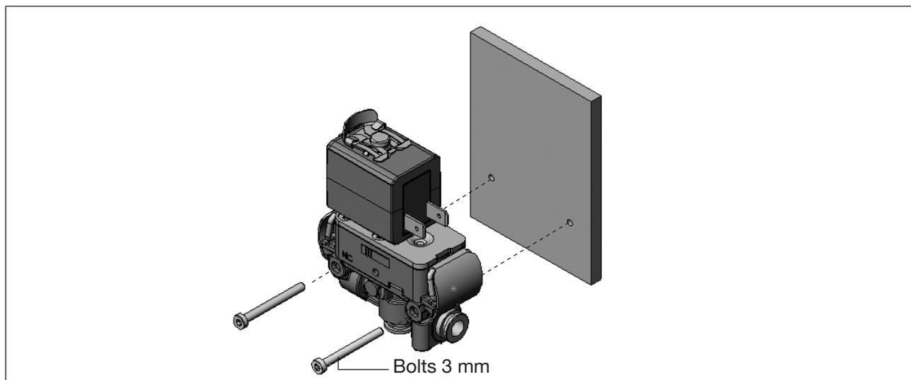
Fig. 5: Horizontal installation of devices with push-in connection
